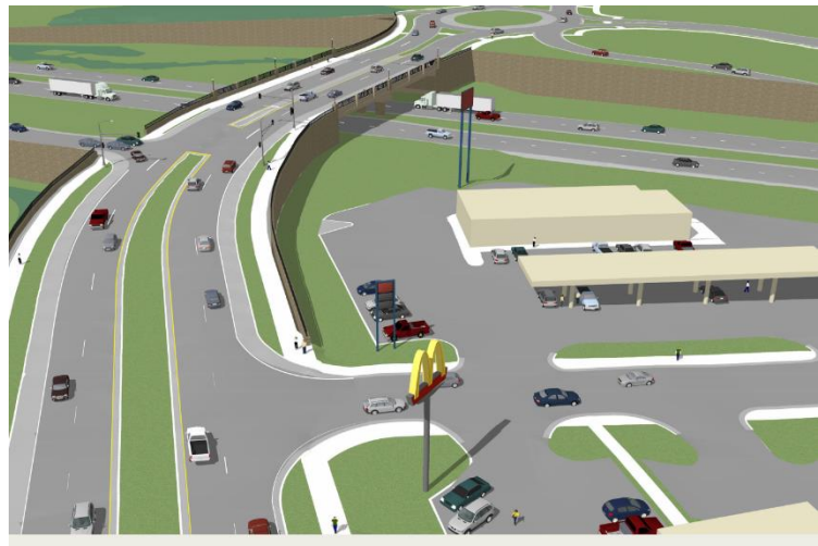
Rendering of the proposed interchange, looking north along TH 282 crossing over US 169 in the City of Jordan
