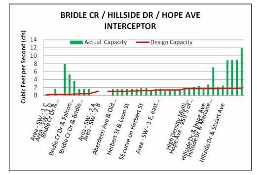
The unused capacities on the ends of the graph represent regions where the sewer is going downhill at steep slopes, which increases the capacity. However, the sewers between Herbert Street and Hope Avenue may require upsizing to avoid backups. Given the improvements in the surrounding area, the cost could be significant.
